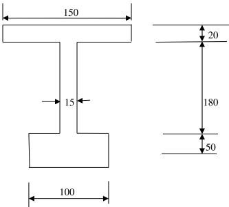
b) Calculate the safe moment of resistance of the beam section shown in the figure in 4 (a) above if the stresses in the upper and lower flanges are limited to 30 N/mm<sup>2</sup> and 20 N/mm<sup>2</sup> respectively.
