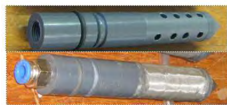
Figure A3.2 (a) A sketch and (b) pictures of the fabricated pore air pressure probe, used in monitoring compressed pore air pressure
