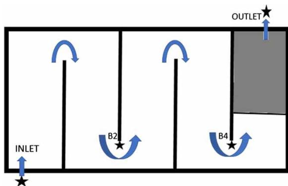
**Figure 1** | A schematic representation of the tropical hybrid CW cell (shaded part is the gravel filled compartment, asterisk represent the sampling points).
