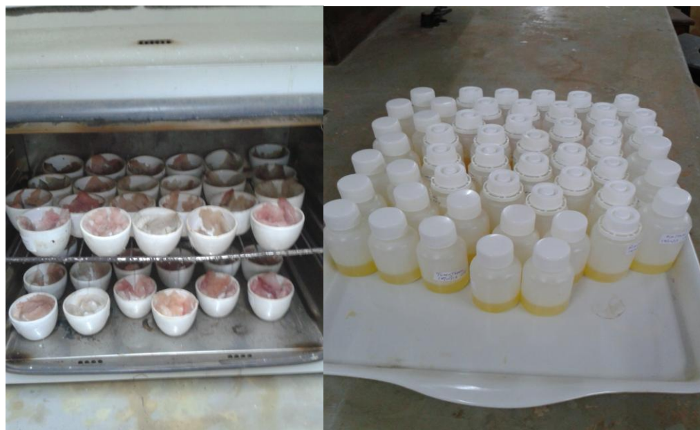
Plate 3.4: Drying of extracted fish muscles and digested fish samples in bottles at the laboratory
