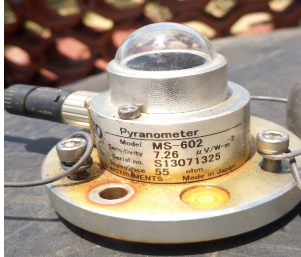
Plate 1: MS-602 Pyranometer used to measure GHI at the site
