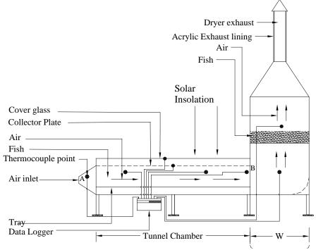
Figure 3: Schematic representation of the solar tunnel dryer
