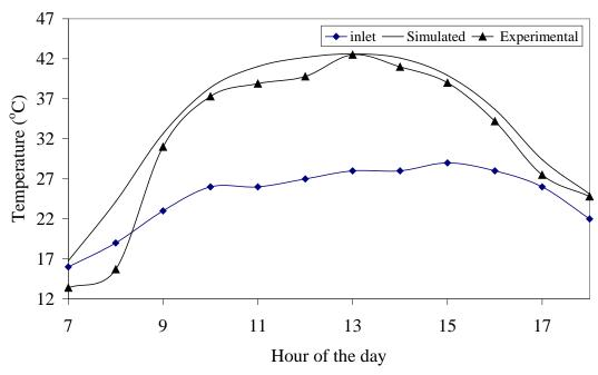
Figure 5: Daily experimental and simulated plenum and inlet air temperatures
