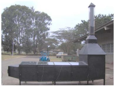
Figure 1: Solar tunnel dryer
