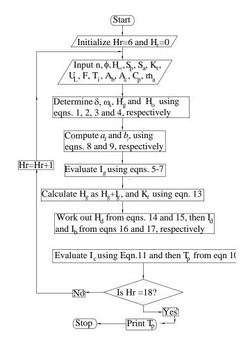
Figure 2: Flow chart for the simulation algorithm
