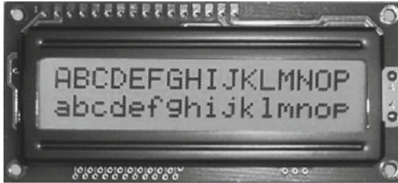
Fig. 8.46 A common 2 × 16 alphanumeric LCD module
