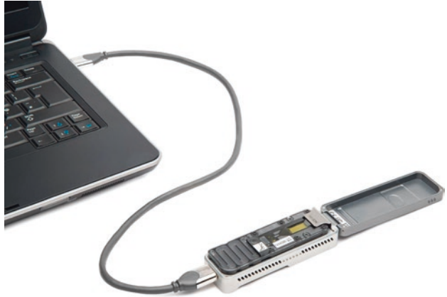
Fig. 3.6 The MinION sequencing device from Oxford Nanopore Technologies (Picture reprinted with permission of Oxford Nanopore Technologies)
