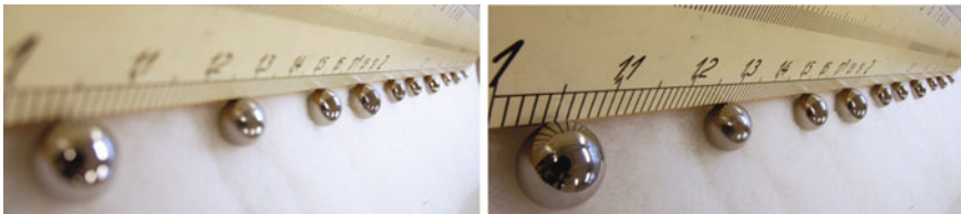
Fig. 12.25 When a luminous point in an object is imaged by a lens, its image will be a point located approximately in the prevailing focal plane. If we are to depict more objects that do not lie at the same distance from the lens, there is no focal plane for the various images that are formed. Then, luminous points in the objects that are at different distances from the lens than the one we have focused on will be depicted as circular discs, and the image will be “blurred”. By reducing the aperture, blurring will be reduced (angle \phi_2 is less than angle \phi_1 in Fig. 12.24) and we say that we have gained greater depth of field. In the photograph on the left, a lens with f-number 3.5 is used with a shutter speed 1/20 s. In the photograph on the right, the same lens and focus are used, but now with f-number 22 and shutter speed 1.6 s
