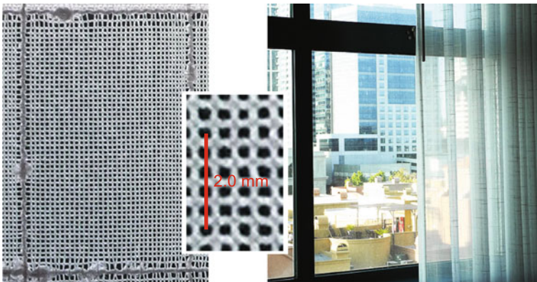
Fig. 13.34 Picture of a light curtain which it was possible to look through. Details show how the fibres in the curtain were in relation to each other. The bar in the middle part is originally 2.0 mm long
