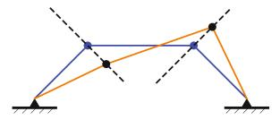
Figure 6.14. Unstable Mechanism of the Three Bar Structure.
