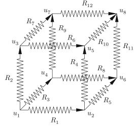
Figure 6.6. Cubical Electrical Network.
