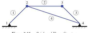
Figure 6.16. Reinforced Planar Structure.
