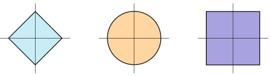
**Figure 3.5.** Unit Balls and Spheres for 1, 2, and  $\infty$  Norms in  $\mathbb{R}^2$ .
