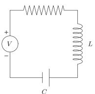
Figure 10.14. The Basic *RLC* Circuit.
