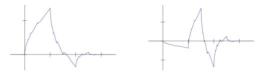
Figure 9.10. The Daubechies Scaling Function and Mother Wavelet.
