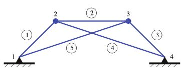
Figure 6.17. Doubly Reinforced Planar Structure.
