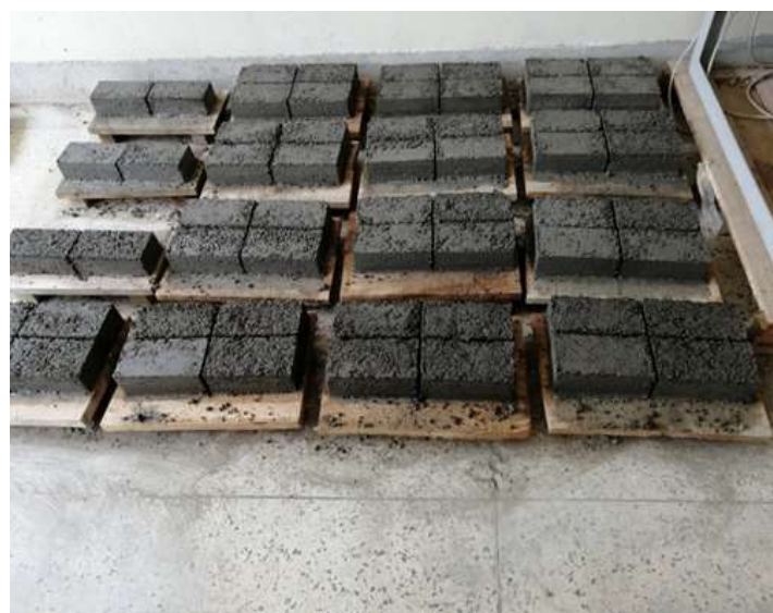
Figure 2: Paving Blocks Before Curing
