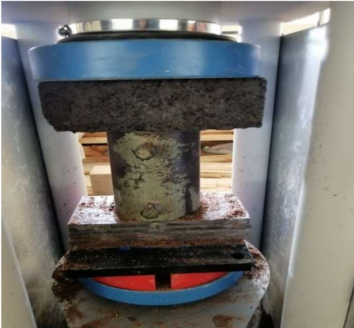
Figure 3: Concrete Sample Under Compressive Strength Test.
