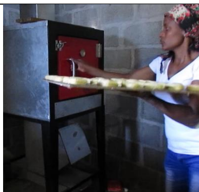
Figure 17: Demonstration of the improved biomass oven during the Dunoon pilot implementation
