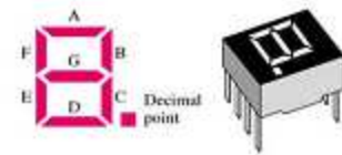
(a) LED segment arrangement and typical device
